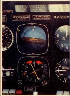
Flight director-autopilot systems such as King's KFC200 (above and right) add airline sophistication to light singles. The KFC200 includes a go-around mode to retrim the aircraft to proper altitude.
