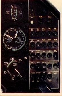
Canted sub-panel on right of instrument panel makes turbine inlet temperature/ compressor discharge temperature and fuel flow/manifold pressure gauges and tachometer easy to read from the left seat.
