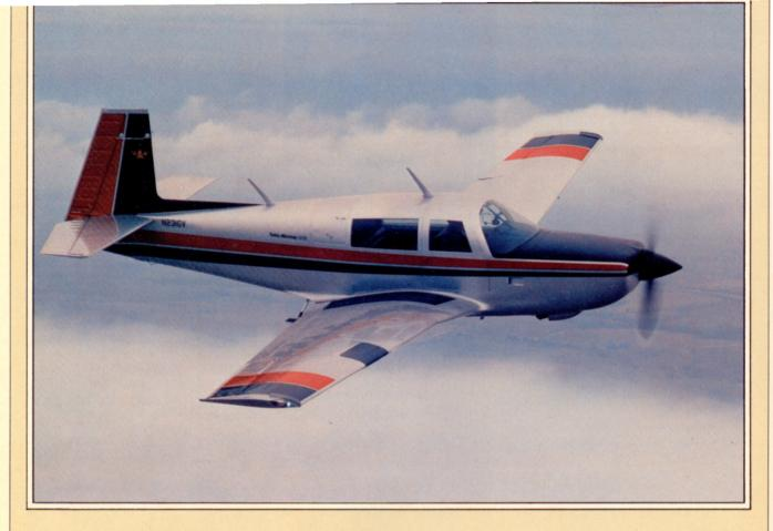
One also has to trade capability for payload. 231GV's 202 pounds of options mean payload with full fuel is 446 pounds. That's two FAA-standard adults plus 106 pounds of other things. Or it requires trading payload for range. More than 70 pounds of the addition to empty weight is from the oxygen system (37.2), radar (26.8) and deicing (6.9) units.
